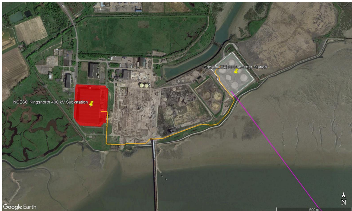
Figure 9 Underground HVDC cable route, converter station site and National Grid Kingsnorth sub-station in UK
