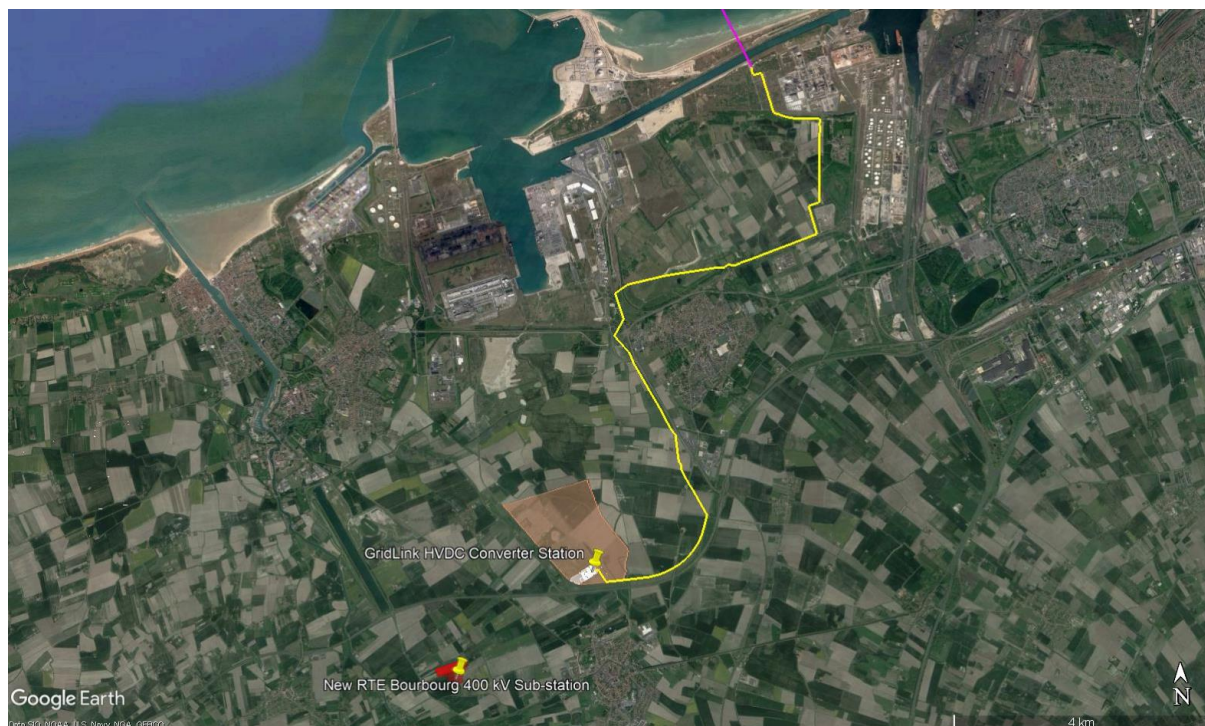
Figure 8 Underground cable route, converter station site and new RTE sub-station in France
