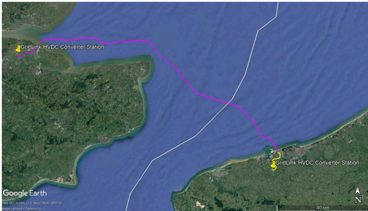
Figure 2: GridLink Converter Station Sites and Cable Route
